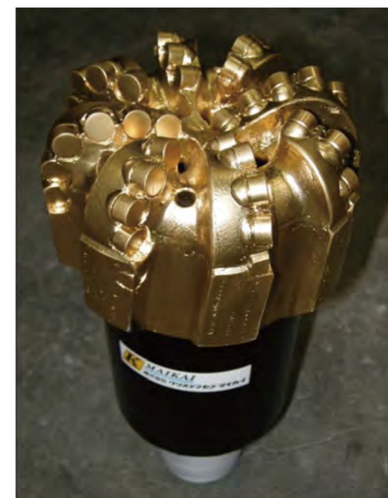
Our prototype (6-1/2 inch PDC Bit)
