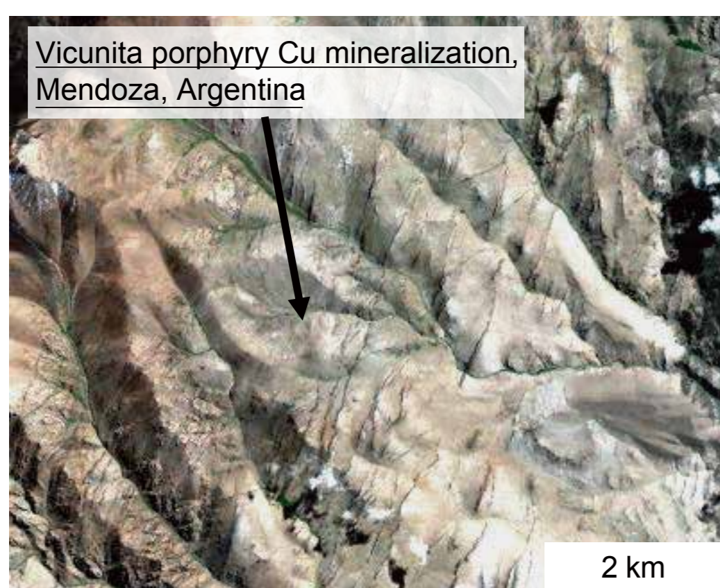
ASTER VNIR false color image (R:G:B=3:2:1). The alteration is not recognizable.
