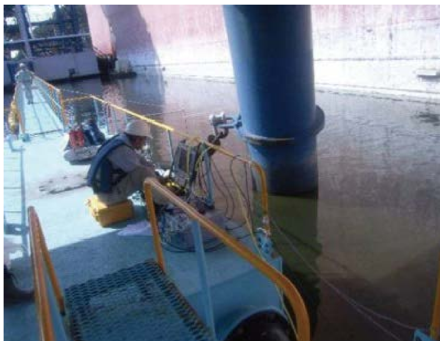
Measuring aluminum anode and shell's corrosion potential
