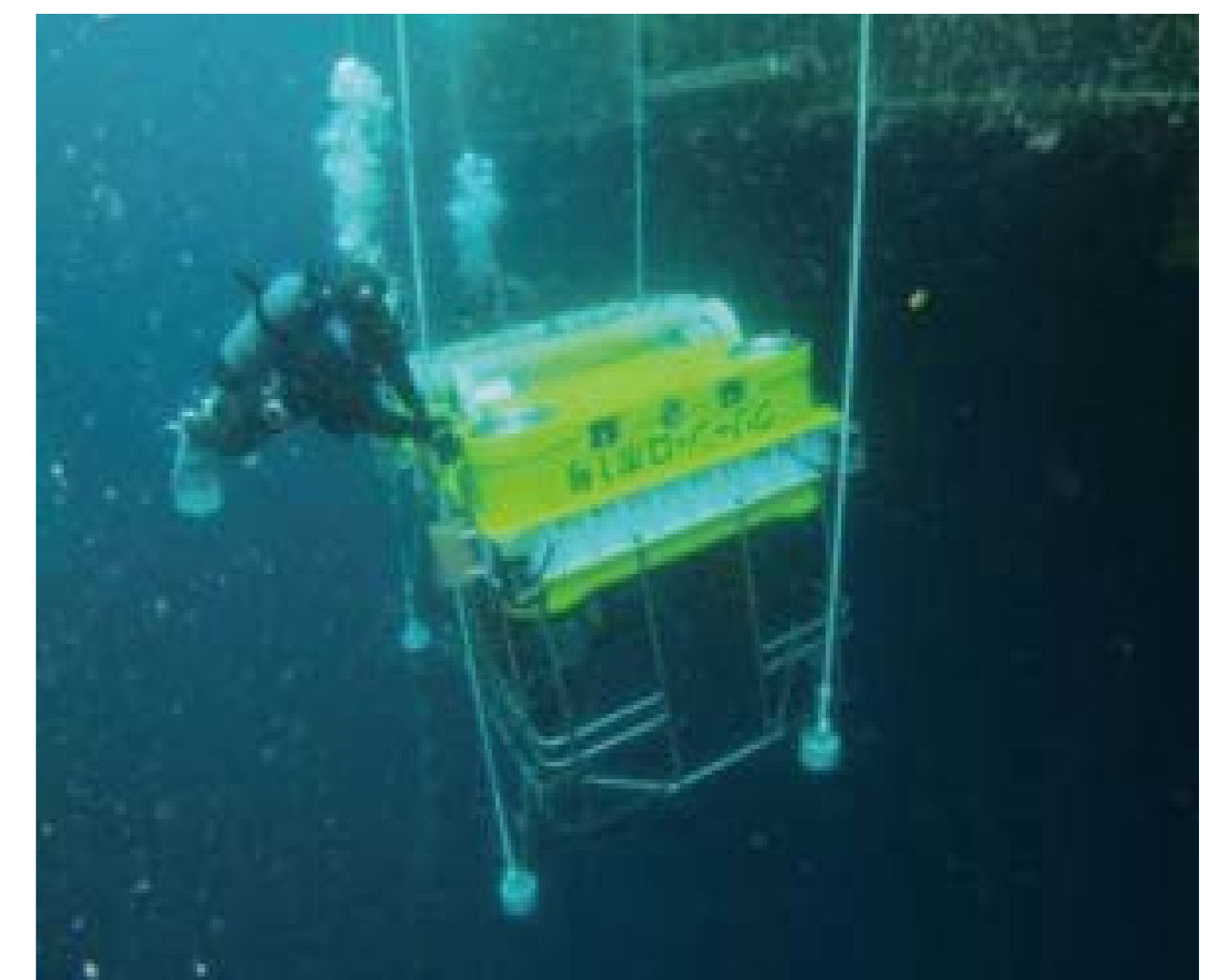
Operating robot under the oil tank
